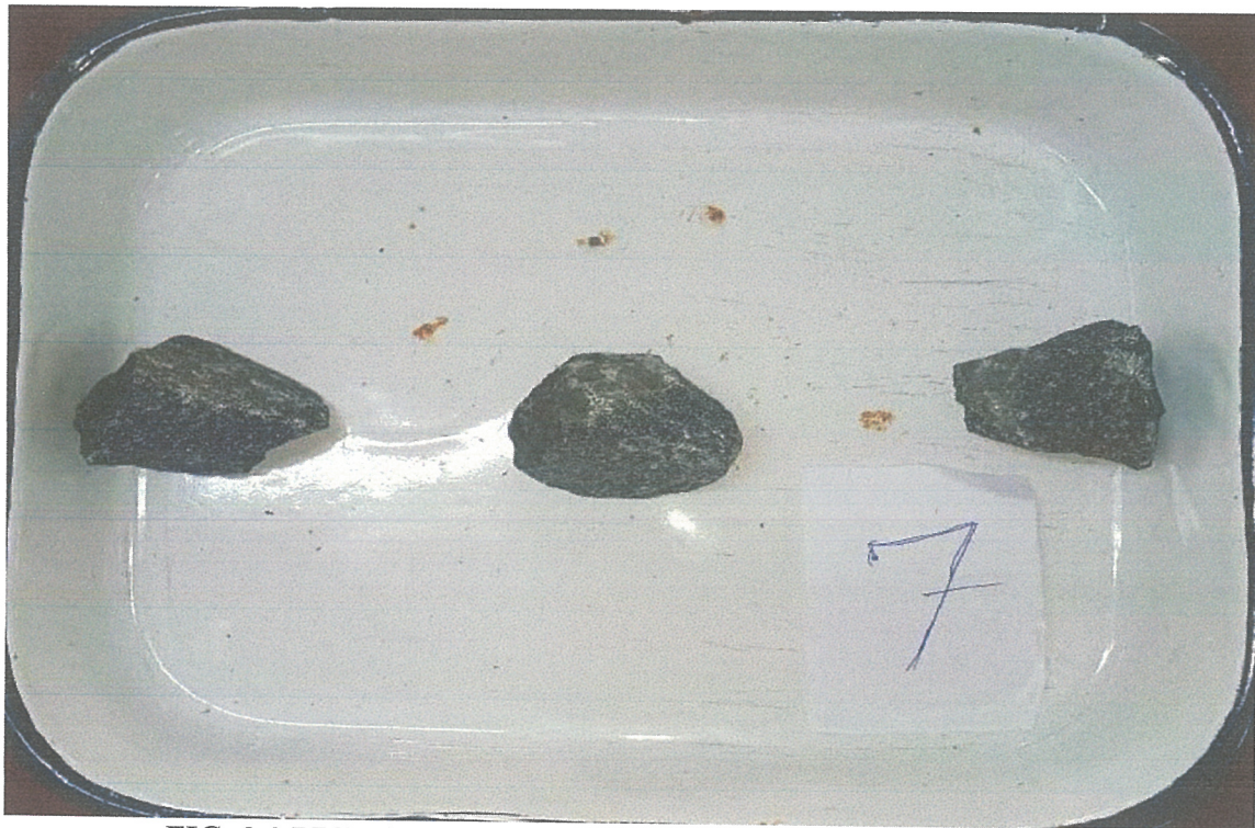
FIG. 2.3 PREPARED SAMPLES TO DETERMINE DENSITY
