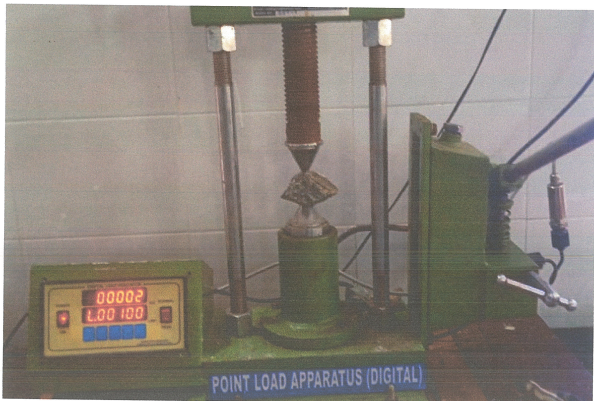
FIG. 2.7 DETERMINATION OF POINT LOAD STRENGTH INDEX
