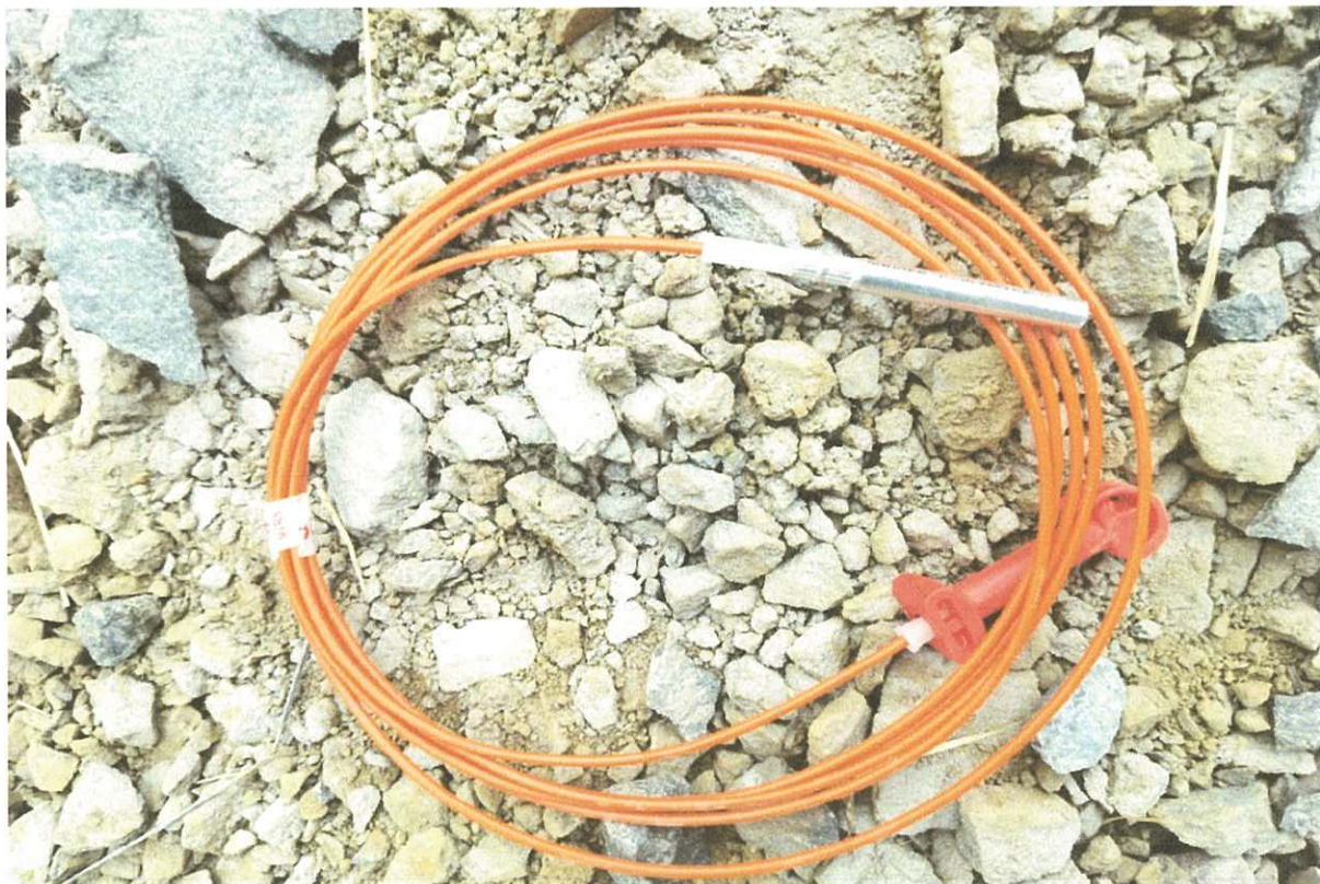
FIG.3.7 A VIEW OF NONEL BASED SHOCKTUBE DETONATORS
