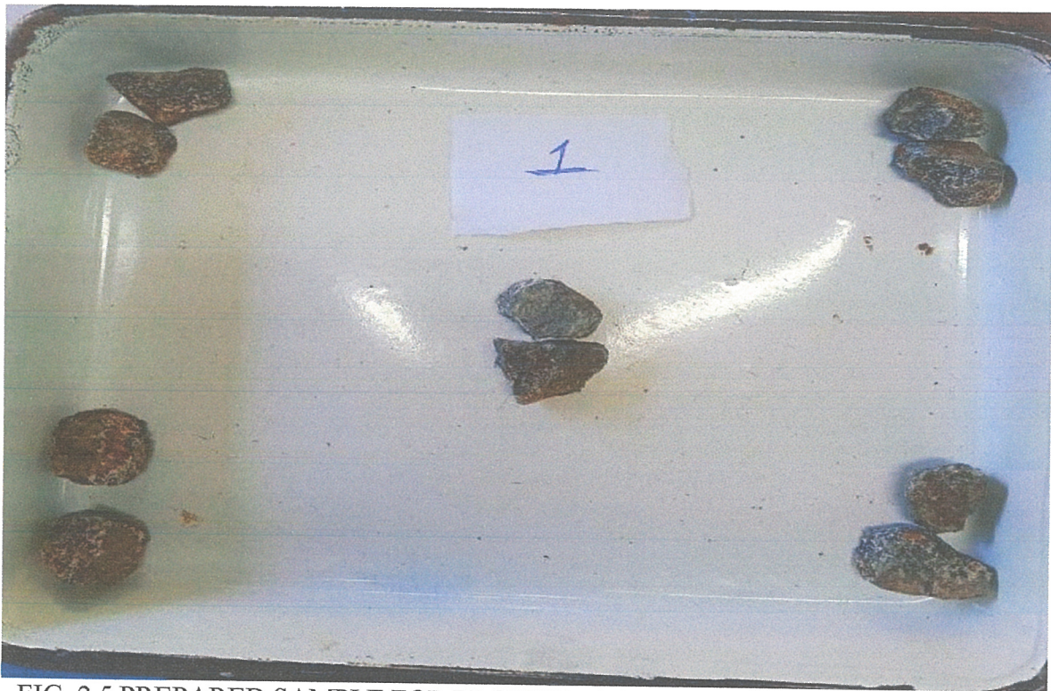
FIG. 2.5 PREPARED SAMPLE FOR PROTODYAKANOV'S STRENGTH INDEX TEST
